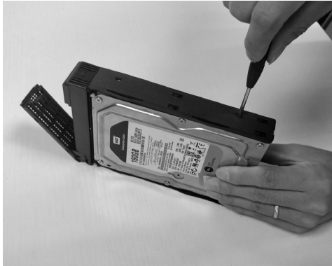
3.5" hard drive(4screws fixed on both sides)
